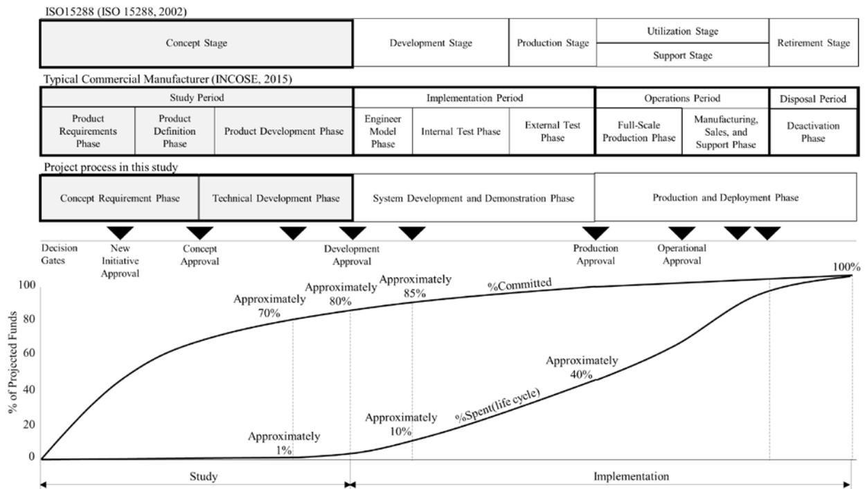
Figure 1. Project life cycle and typical expenditure profile (INCOSE, 2015), added project process in this study by the author
